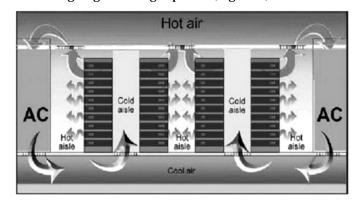
Figure 3: Typical air flow in a traditional data ceneter.
