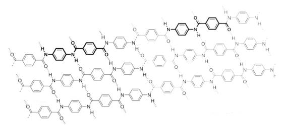
*Figure 2: The monomer unit of Kevlar is outlined in bold. The crosslinks between the polymers is indicated by dotted lines.*
