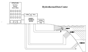
Figure 4: The above illustrates the concept of a large data center using tunnel boring and directional drilling to access and discharge cold and warm seawater or lake water. The cold water will be used for cooling the data center. Turbines and heat exchangers will generate clean electric power by utilizing the temperature difference of warm surface water and deep cold water. This power is used to
